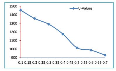
Figure 1: Variation of ultrasonic velocity with mole fraction
